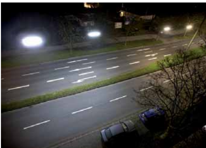
Comparison of street lighting products front: HERNE, rear: conventional luminaire
