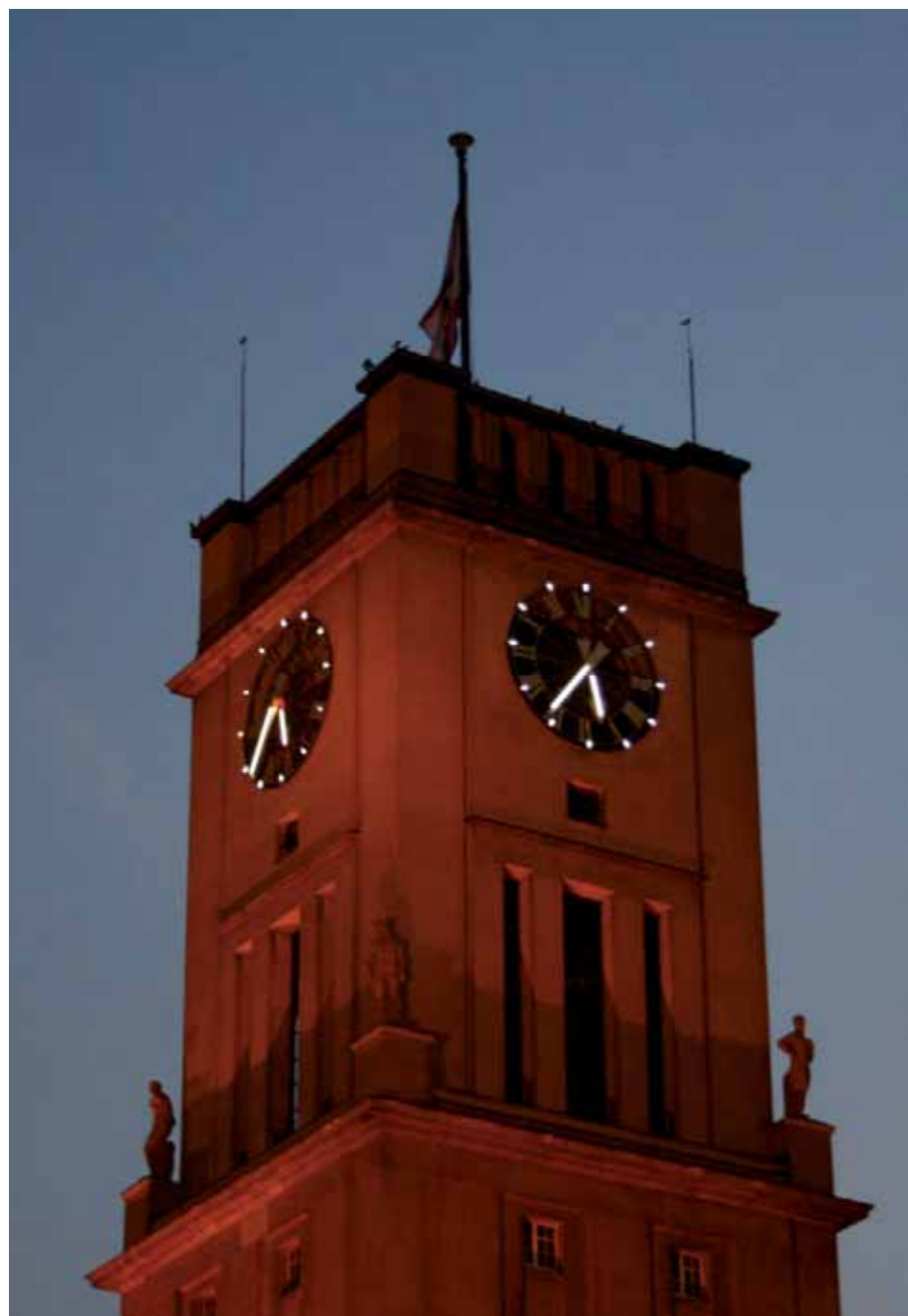
LUZERN 16 LED tubular luminaire, 24 V DC, 80 lm/W, beam angle 120°, 5400 K, tube in PMMA, clear, with 5.0 m connecting cable
